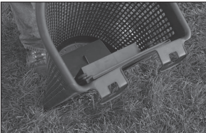
Fig. 30 Use 6 small stainless screws threaded in from outside face of the basket to attach the slide assembly.
