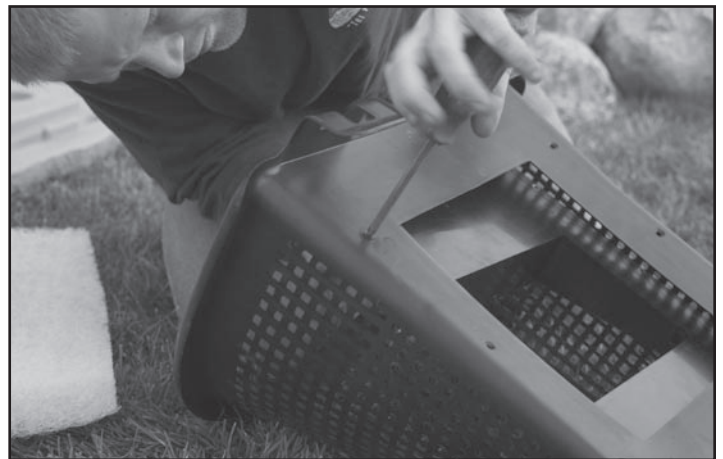
Fig. 29 Place the slide assembly inside the basket.
