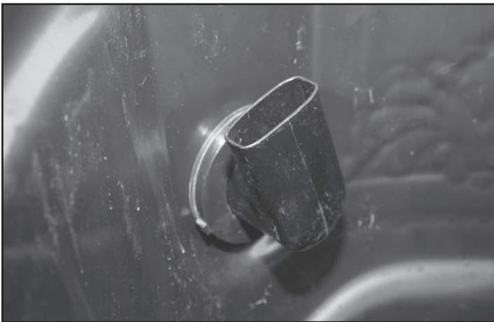
Fig. 33 Dial-in the adjustable overflow arm.
