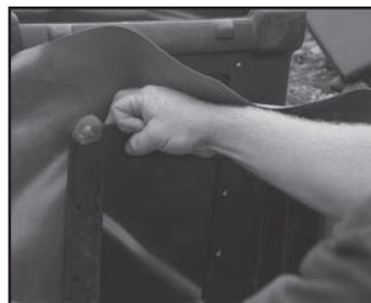
Fig. 14 Remove the awl or nail while holding the liner plate and liner in place and begin threading one of the screws into the filter.
