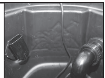
Fig. 10 Single pump and overflow.
